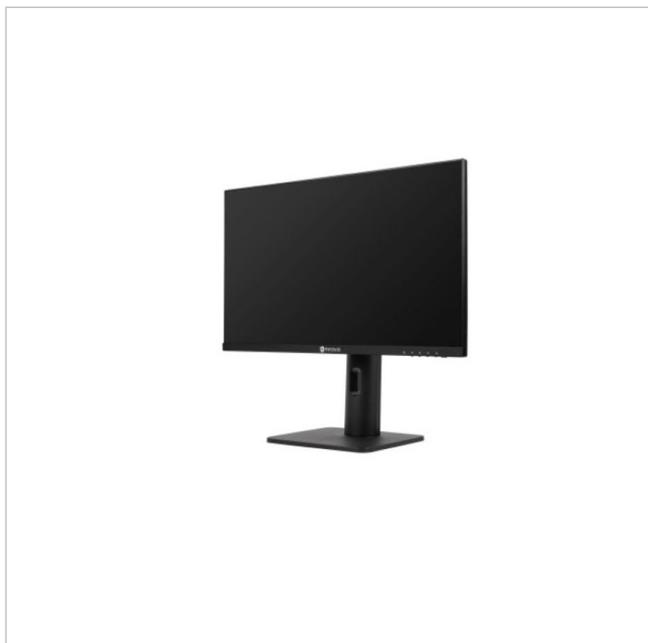
27" (68,6cm) LCD Monitor, LED, 1920x1080, HDMI, VGA, DisplayPort, Audio
